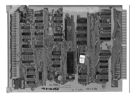
Locate the EPROM card (it should be the only card without any cables attached to the end). Press the release levers on the EPROM card and remove it as well. The EPROM card for different games will have different numbers of chips on it. It will look something like this:
